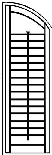
**Solid-Top Arch** Maximum rise is 15 inches from the break. Maximum overall width 96". Quote for 5 panels and up or widths wider than 96"
