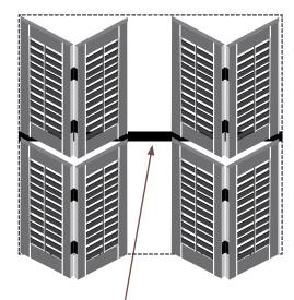
Horizontal T-Post Ex.) Double Hung Panels with horizontal T-Post
