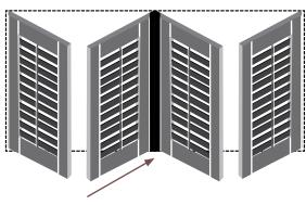
**Vertical T-Post** *Ex.)* Four panels with one vertical T-Post
